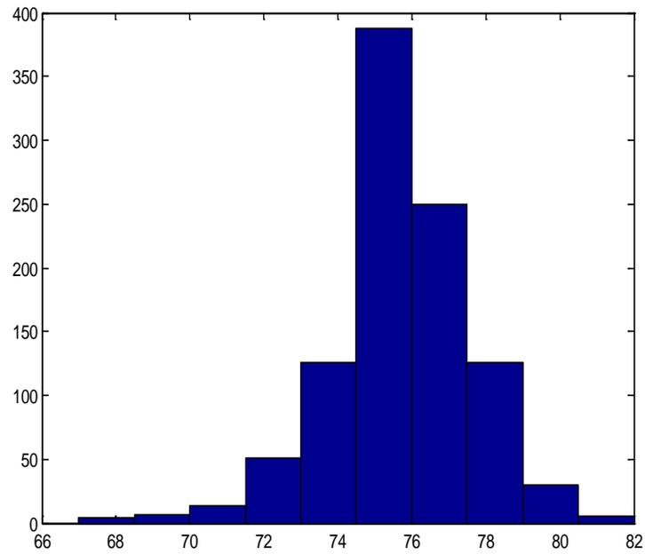
Figure 4. Number of randomly located tows in a fixed time with the minimum track obtained using the travelling salesman algorithm. (9 days with a survey speed of 10 knots and trawling time of 1.5 hours in a 14,400 N.mi<sup>2</sup> area) This compares with a systematic grid of 64 tows in the same time period.
