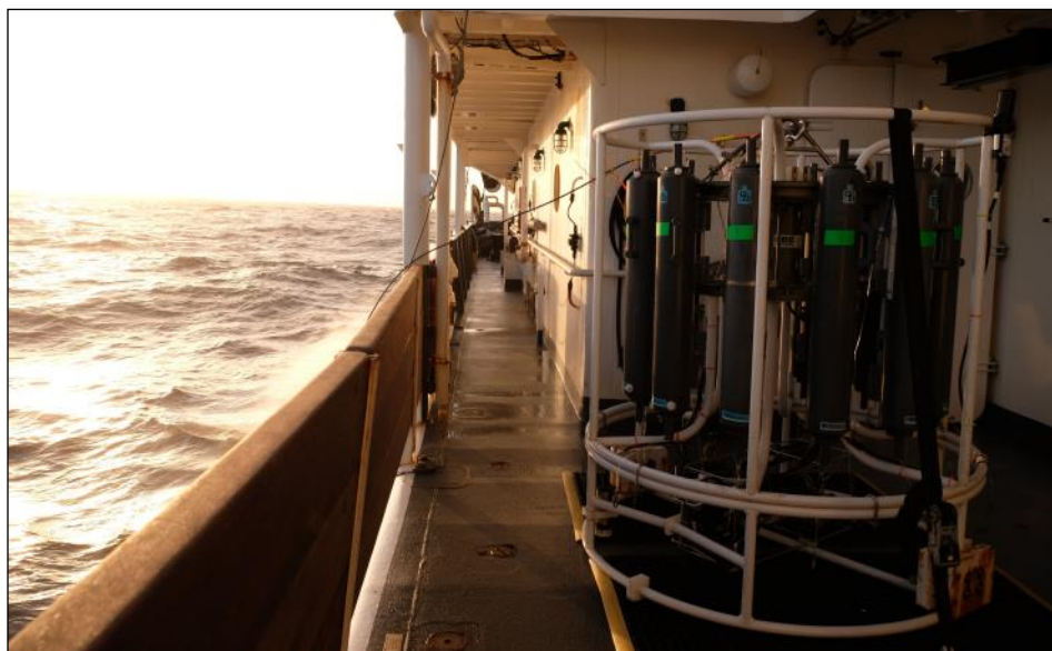
A CTD rosette (a scientific instrument used to measure properties of seawater, primarily conductivity, temperature, and depth) on the Reuben Lasker. (Photo Corey Ridings)
