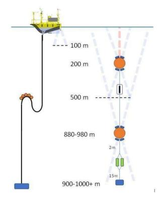
The subsurface current profiler system will be located at WGS84 41° 06' 15.8" N, 124° 40' 00.1" W on a taut mooring with no surface presence and a clearance depth of 200 m over the upper float. The deployed systems will be listed in the USCG Light List, Notice to Mariners, and updated charts upon deployment.
