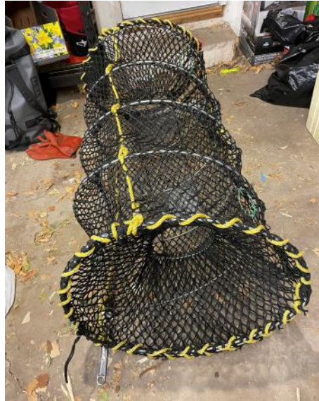
Slinky pot example. Photo: Fish Tech Inc.
