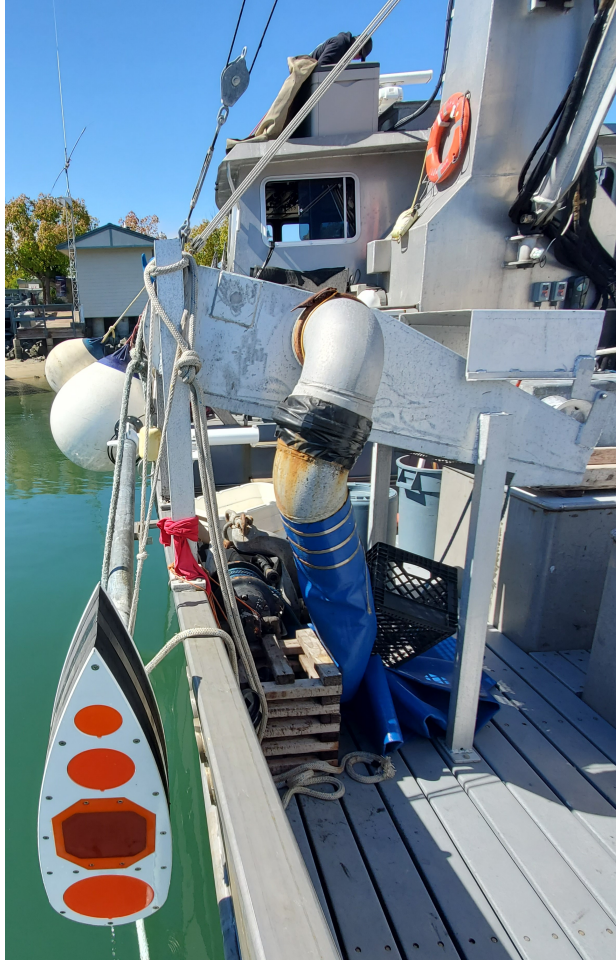
Figure 5: Transducer locations on the bottom of the pole-mounted multi-transducer array (MTA4) installed on the F/V Long Beach Carnage .
