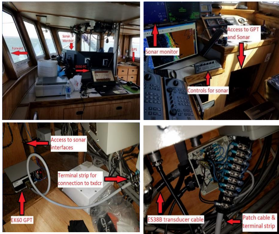
Figure 1. The bridge of Lisa Marie where the EK60 controlling and logging laptop is located. A table located to the port side of the helm station, behind the array of instrumentation and monitors (top left); the EK60 GPT and Furuno CH-250 sonar transceiver installed under the main console in the wheelhouse (top right); the EK60 GPT attached to the deck with Velcro (bottom left); and the transducer patch cable connected to the transducer through a terminal strip in a junction box (bottom right).
