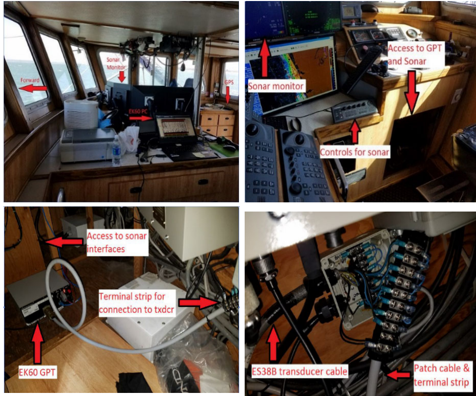
Figure 11. The bridge of Lisa Marie where the EK60 controlling and logging laptop is located. A table located to the port side of the helm station, behind the array of instrumentation and monitors (top left); the EK60 GPT and Furuno CH-250 sonar transceiver installed under the main console in the wheelhouse (top right); the EK60 GPT attached to the deck with Velcro (bottom left); and the transducer patch cable connected to the transducer through a terminal strip in a junction box (bottom right).
