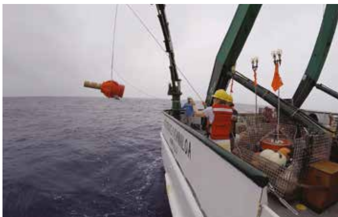
A deep Sounding Oceanographic Lagrangian Observer (SLO) float deployment off the R/V Ka'imikai-O-Kanaloa during a Hawai'i Ocean Timeseries (HOT) cruise in the Pacific. Photo credit: Blake Watkins, University of Hawai'i (May 2019)
