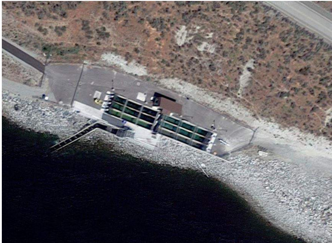
Figure 7-9. Aerial view of Chief Joseph Hatchery adult fish ladder. The fish ladder is located on the right bank 0.5 miles downstream of Chief Joseph Dam.
