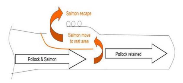
Figure 9: Flapper whiting excluder that has had limited success in Alaskan pollock EFPs, especially for smaller vessels with lower horsepower.
