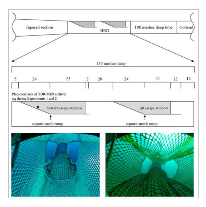
Figure 10: Schematic diagram of the open escape window BRD tested in Experiment 1 and 2 (top); forward view of the forward set of escape windows under ambient light (bottom left image); forward view of the aft set of escape windows under ambient light (bottom right image). Note: diagram not to scale. From Lomeli and Wakefield (*in press*).
