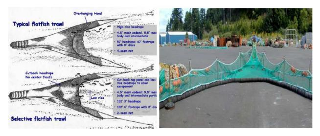
Figure 6: Comparison of SFFT vs traditional hooded trawls, which demonstrates why the cut-back headrope of SFFT that allow salmon to swim up-and-over are an effective means for reducing Chinook salmon bycatch. The headrope height (i.e., vertical opening) is also lower for the SFFT than for most hooded trawls (see Table 3-19 in Final Environmental Assessment Trawl Gear Regulations).
