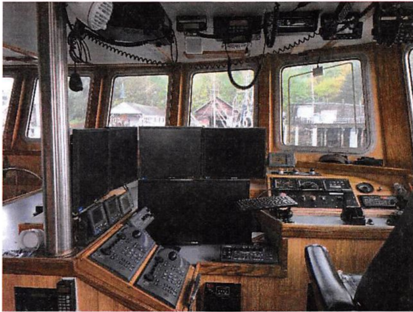
Figure 8. Table on the bridge of Lisa Marie (left) where the EK60 GPT, laptop, and sonar- display recording equipment will be located. The table is located to the port side of the helm station, behind the array of instrumentation and monitors (right).
