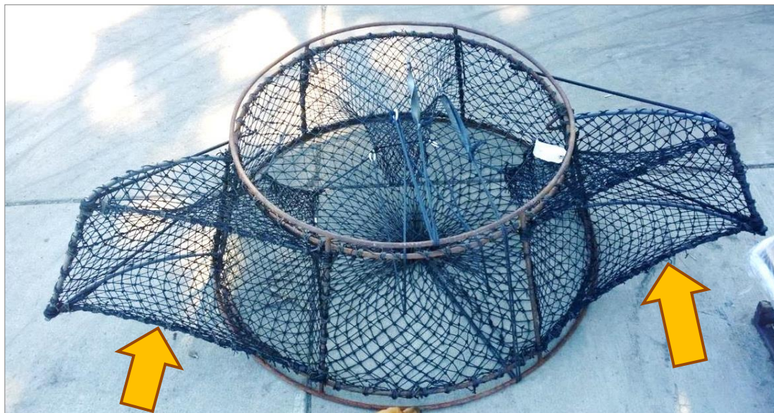
Figure 2. Collapsible-wing pot for EFP testing. Arrows indicate entry points for fish. Escapement ring not shown.
