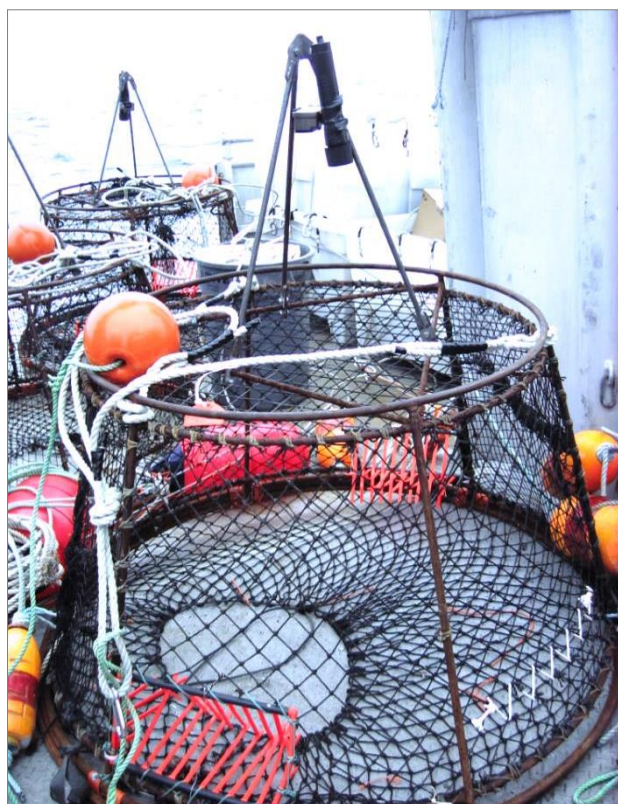
Figure 3. Trigger pot gear with top-mounted camera on deck of F/V Morning Star. Preliminary gear testing, June 2014.
