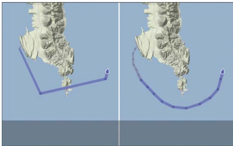
Figure 1-1. Schematic of vessel track. Left panel is one hour ping rate, right panel is one minute ping rate.
