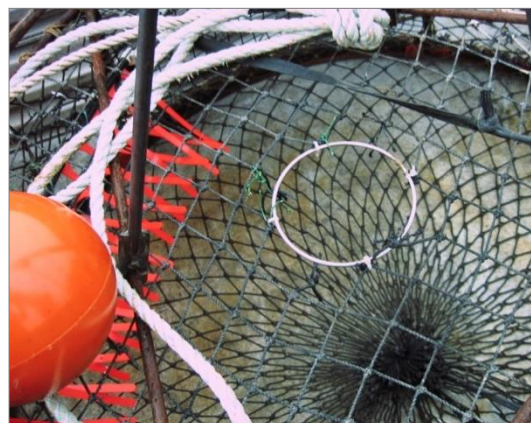
Figure 4. Aluminum escapement ring mounted in top webbing of trigger pot. Preliminary gear testing, June 2014.
