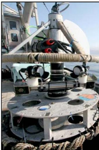
**Figure 4.** Rotating stereo-video lander system designed for conducting visual surveys for this project.
