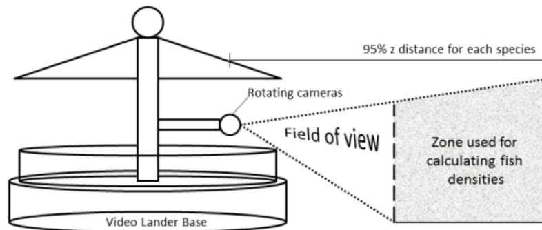
**Figure 5.** Geometry of the field of view and area used for density calculations for the stereo-video lander.
