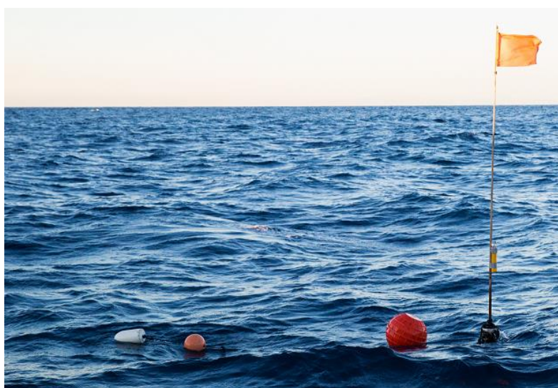
Figure 2. A set of DSBG showing the strike detection system at work. In this image, a swordfish is on the line resulting in the presentation of the white strike indicator at the surface.
