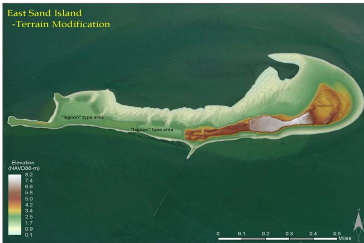
FIGURE 2-4. Proposed terrain modification, creating "lagoon" type areas in the DCCO nesting area on the western portion of East Sand Island.
