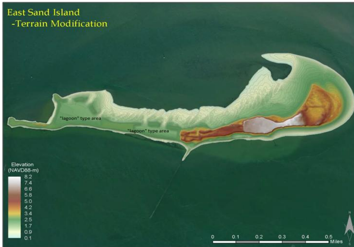
FIGURE 5-2. Proposed terrain modification, creating "lagoon" type areas in the DCCO nesting area on the western portion of East Sand Island.
