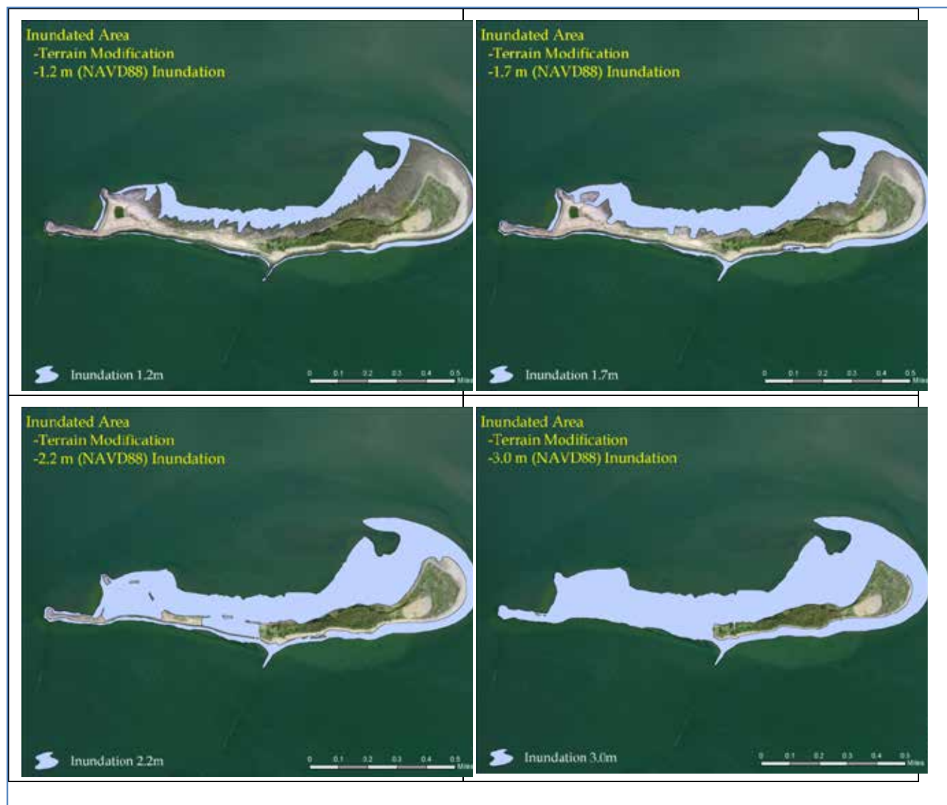
FIGURE 4-1. Water inundation outputs from the ATIIM for the terrain modification, representing four surface elevations: 1.2, 1.7, 2.2 and 3.0 m (NAVD88).
