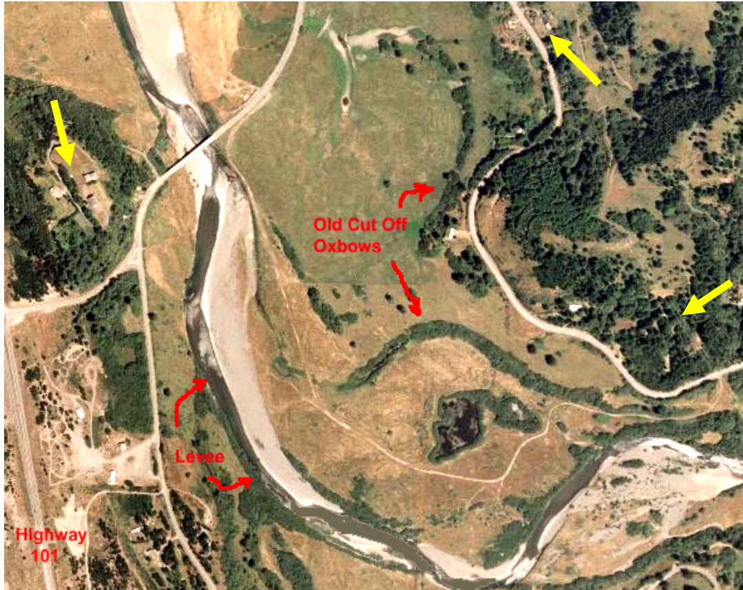
Figure 12-3. Aerial photo of Pistol River showing confinement by a levee. The levee separates the active channel from adjacent farm and industrial gravel operation to the west (left). The levees also cut off the river from oxbows and meanders on the east bank (right), which would have formerly created ideal coho salmon rearing areas. Yellow arrows highlight pockets of residential development.
