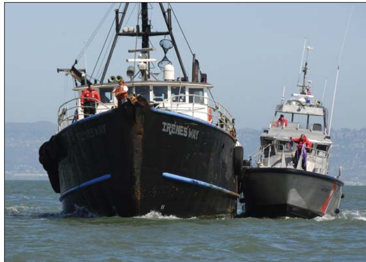
A 47-foot motor lifeboat crew, from Coast Guard Station Golden Gate, performs a side tow of the F/V Irene's Way March 13, 2009. The lifeboat crew towed the over 75-foot fishing vessel after the skipper reported the vessel was disabled just outside the Golden Gate Bridge. (Photo: U.S. Coast Guard/Erik Swanson)
