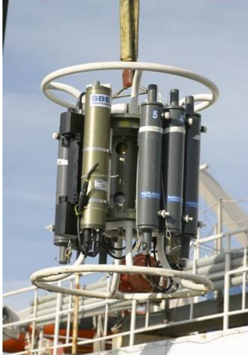
Figure 24. Water quality data can be collected by lowering electronic monitoring equipment into the ocean to sample a water column profile. The rosette is a series of instruments and sampling chambers on a metal frame, that measure temperature, pressure, salinity, oxygen content, algae content, and other factors. (Photo: Olympic Coast sanctuary)
