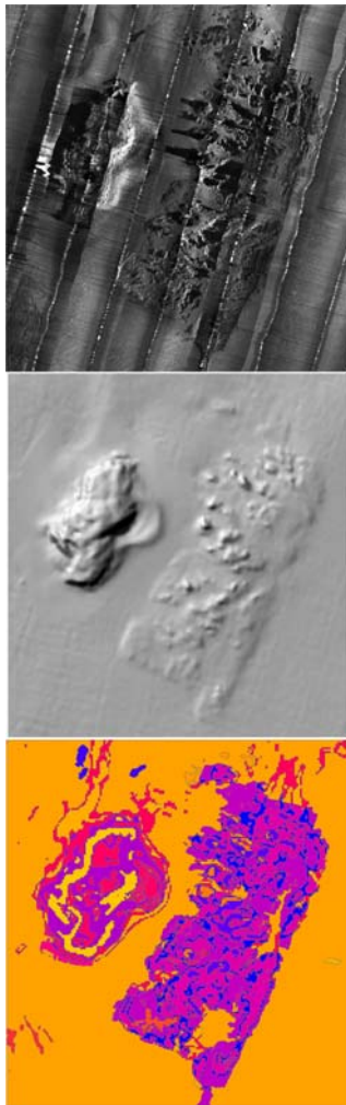
Figure 20. Using texture analysis algorithms, information from side scan sonar imagery (top plate) and multibeam bathymetry (middle plate) are combined to create classified habitat images (bottom plate). (Image: Olympic Coast sanctuary)
