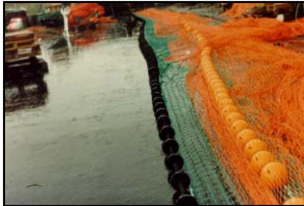
Figure 4: Photograph of a trawl net with orange floatline and black rubber footrope gear. (courtesy of Christopher Kubiak)
