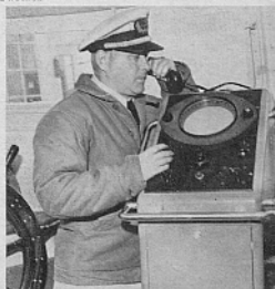
• Radar and radio-telephone help Captain Ralph Dale locate suspicious craft at night or in fog
