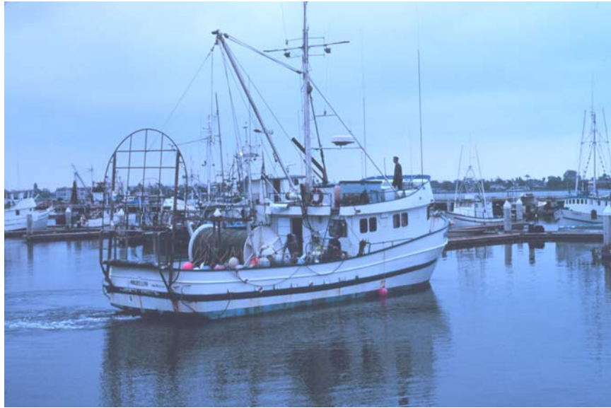
Figure 3.4. A southern California DGN vessel showing net reel and stern grate. (Photo: NOAA Fisheries Photo Library.)
